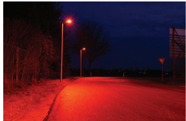
Figure 21: Red, bat-friendly streetlights along the A4440 have less adverse impacts than white lights (by Worcestershire County Council)
