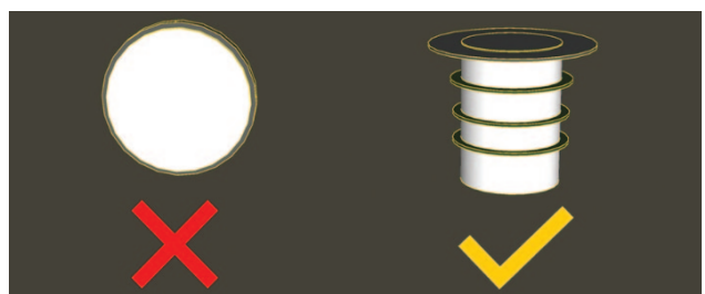
Figure 10: Avoid globes and bulkheads, which provide no control over the direction of light
