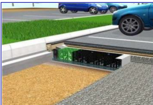
Figure 3 Geocellular system under a car park
