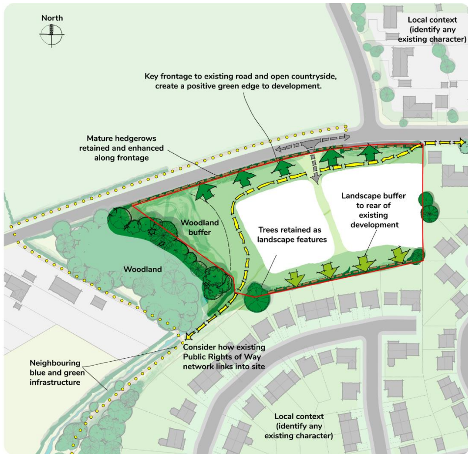
Figure 3a: Identify, retain, and enhance the green infrastructure and natural features as part of a scheme (minor example)
