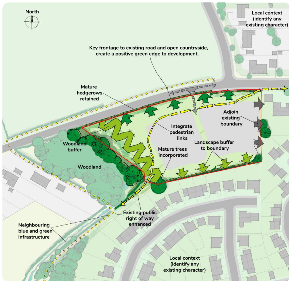
Figure 2a: Develop a design rationale based around the site's features, opportunities and constraints (minor example)
