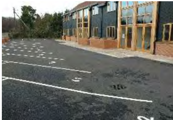
Avoid large expanses of a single surfacing material, this could have been broken up with alternative materials and more planting. (Penn Street)
