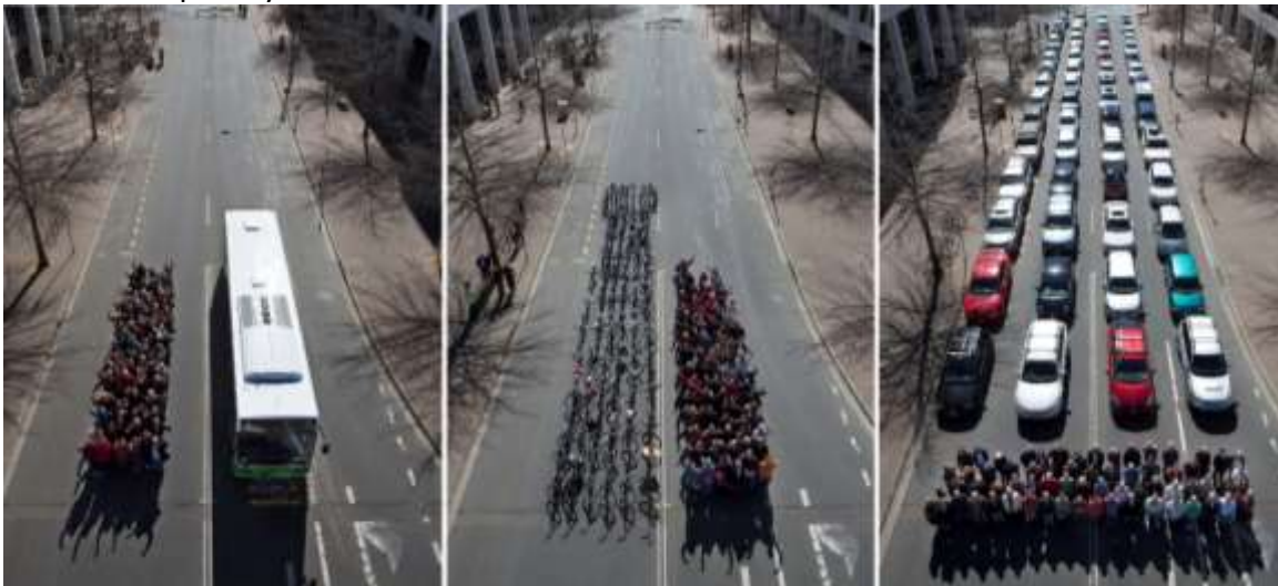
Figure 24 – Street space required to accommodate 60 people by bus, bicycle and car 49
