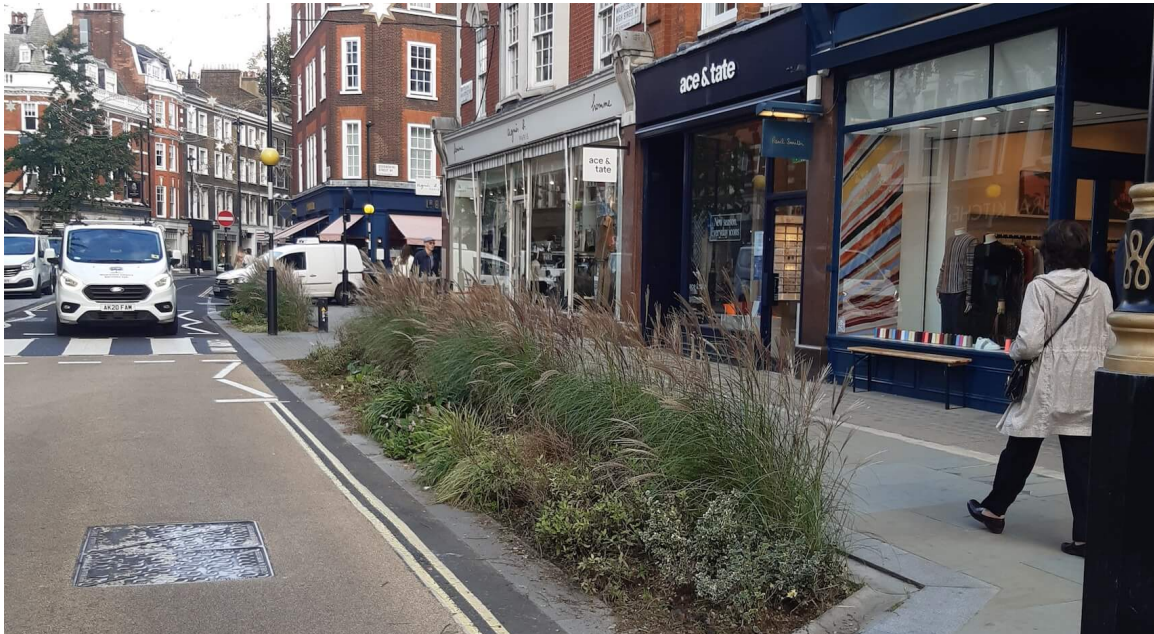
Figure 29: Example of raingardens integrated into an existing street
